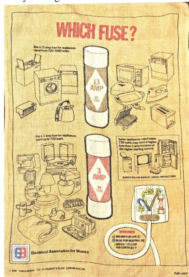
Fig.10 An EAW Tea Towel describing which fuse to use for each appliance in a fused plug.
