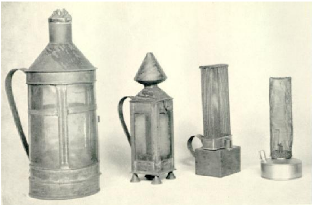
Some of Davy's own experimental models of the Miners' Safety Lamp
